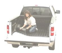
With ribbed side up and with the mat part number visible on the lower right side of the truck bed, lift the mat into the truck bed. Begin tucking the mat into the channel on one side of the bed and repeat for the opposite side. Make sure the mat is pulled tightly to the front of the truck.
