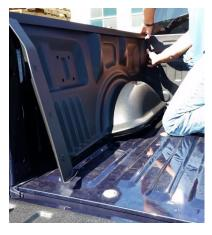
If your truck is equipped with LED lights, there are pre-cut holes for both lights and the switch. If your truck is equipped with a bed extender, you will see three pin marks at the back edge of the side panel that aligns with the holes for your bed extender. Open these up to
