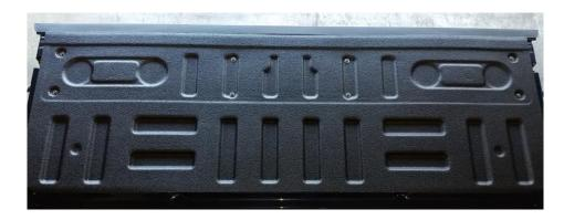
For added security we've included Christmas tree pins. Should you want to secure the panel better, you can drill ¼" holes in the center of the two circular recesses on the lower half of the tailgate and between the cup holders on the top half. Lift the panel to clear away any chips from drilling. Apply rust preventative to each hole and to the Christmas tree pin. Insert one pin in each hole, twisting the pin to evenly distribute the rust preventative.
